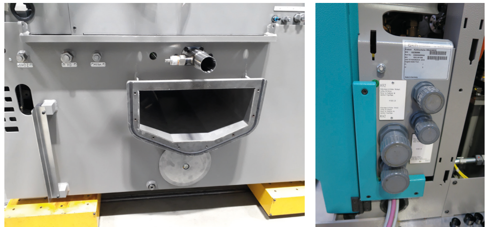
Illustration 01 and 02: mechanical and fluidic connection points at a multi-spindle turning machine
