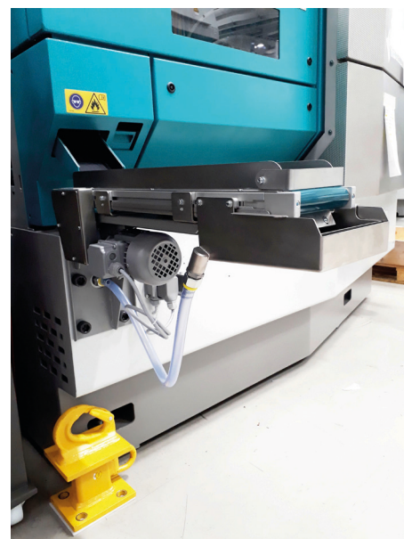
Illustration 02 and 03: Example MS40-6 equipped with external conveyor belt
