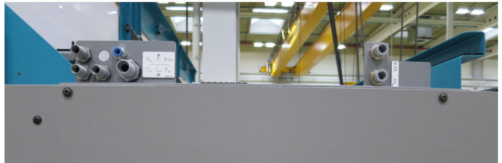
Illustration 01: Example: fluidic connections at an MBL-bar loading magazine.
