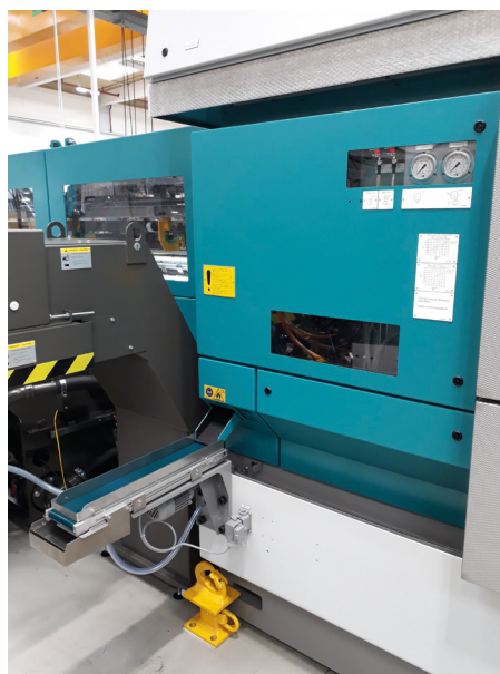
Illustration 02 and 03: Example MS40-6 equipped with external conveyor belt
